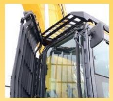
Hinged front guard to allow easy access for windscreen cleaning. The Demolition Safety SpaceCab<sup>™</sup> is ROPS compliant with ISO 12117-2:2008.
