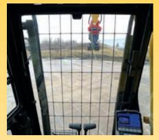
Carefully aligned grid layout ensures maximum visibility with correct protection. One piece front screen fitted with high impact protective glass.
