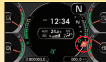
AdBlue® level gauge and refill guidance
