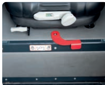
Work equipment safety lock lever
