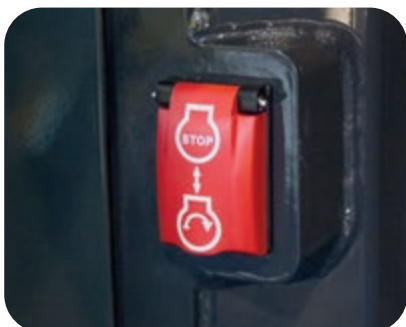
Secondary engine shutdown switch
