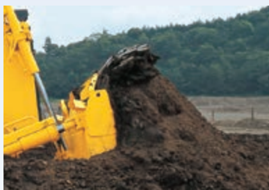
The Sigmodozer® blade offers highest material holding capacity
