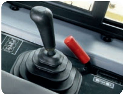
Remote safety lock levers
